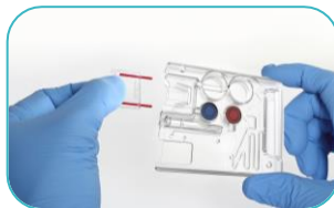
Insertion of sampler into modular cartridge integrated with reagents
